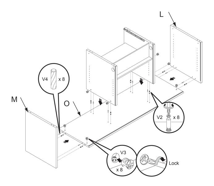
5. Place the assembled center part onto the top board(O) first with screws(V2)and cam lock(V3). Attach main side board (M & L) to the top board (O) with screws (V2),cam lock(V3) and wooden dowels (V4). Turn the CAM lock(V3) clockwise to secure.
